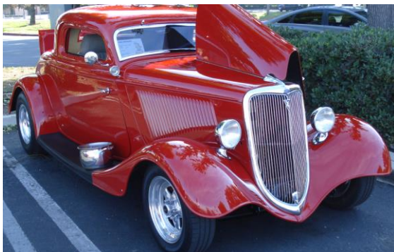
Front wheel drive early Merc custom dropped on a 1998 Buick chassis
