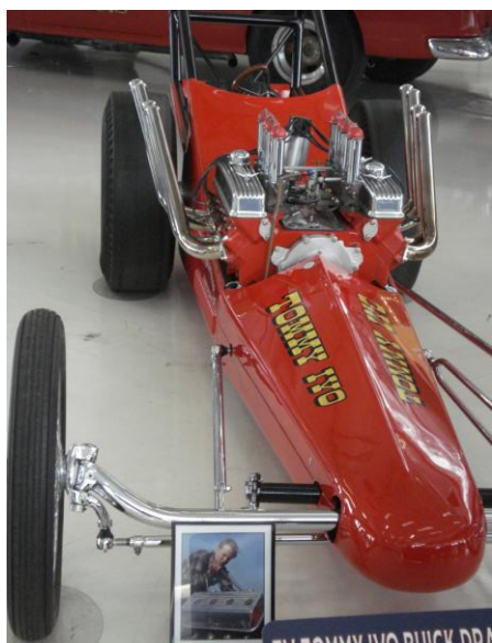
1958 TV Tommy Ivo Buick powered dragster set a world record of 9.50 seconds at 141.38 mph on gas
