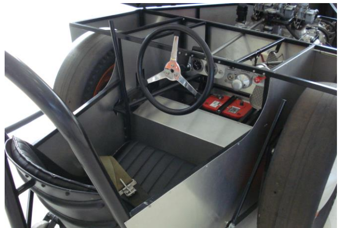
"Slice-O-Pie" dragster from 1955, Flathead V8 powered with chain drive to rear wheels
