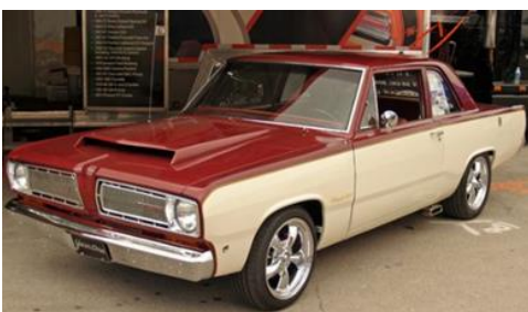
1968 Plymouth Valiant give away car built by Inland Mopars in 2008 to benefit CSDR. 400CI, 727, Reilly Motor Sports AlterKtion front end, Legendary Interior installed by Ron Mangus.
